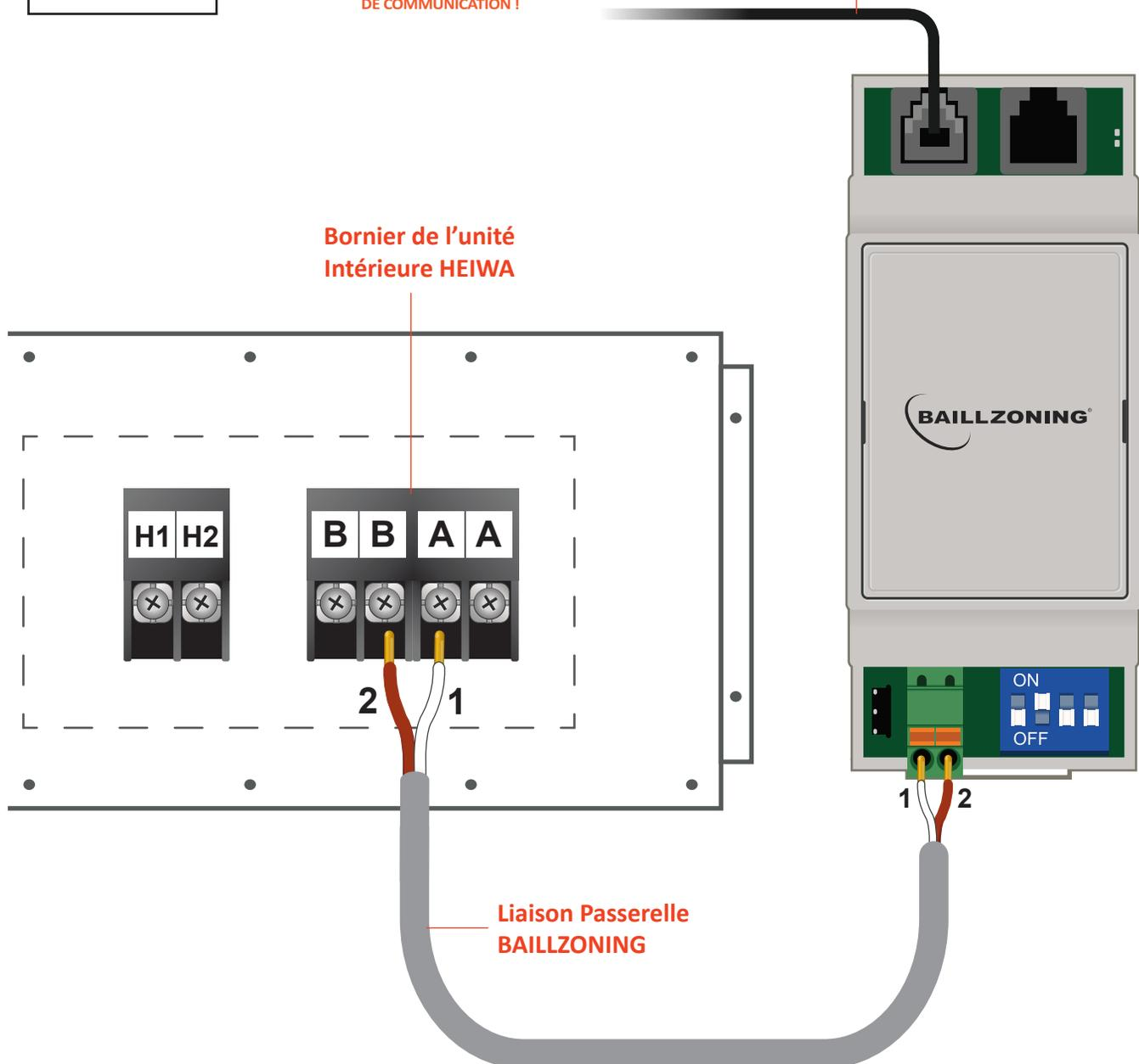
**NE PAS BRANCHER LA TELECOMMANDE GREE EN PARALLELE AVEC LA REGULATION BAILLZONING !**
